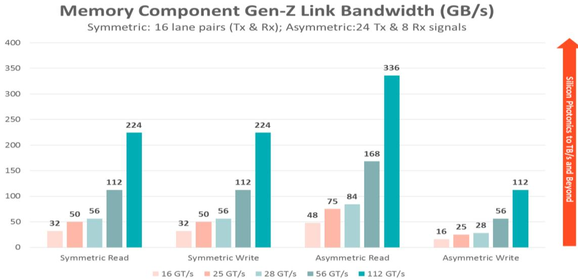
Figure 4: Examples of Gen-Z Memory Component Link Bandwidth
