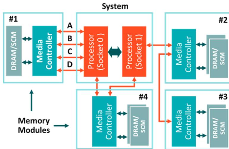
Figure 5: Gen-Z Enables Memory Subsystem Design Flexibility
