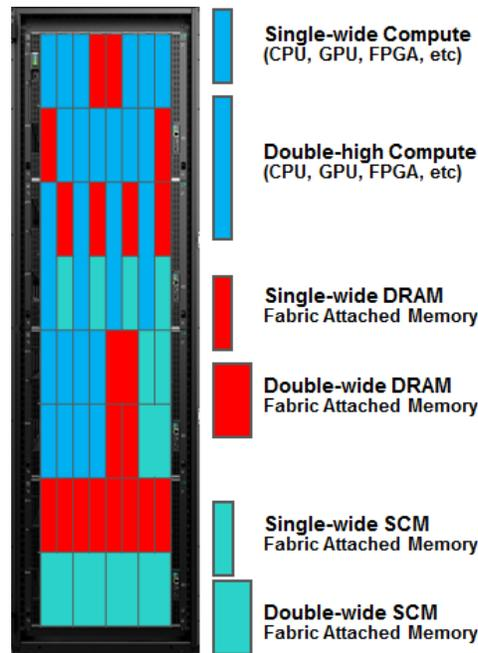
Figure 10: Example: Rack-scale Fabric Attached Memory Deployment
