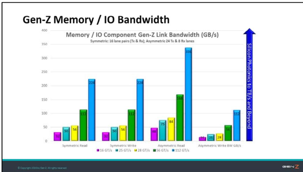
Gen-Z supports multiple signaling rates that when combined with a variable number of transmit and receive lanes, can scale to meet demanding application needs. The bandwidths shown can be achieved using electrical or optical physical layers. Long-term, as silicon photonics evolve and start to displace electrical, Gen-Z's architecture will enable solutions to scale bandwidth to multi-Terabyte/s ranges.
